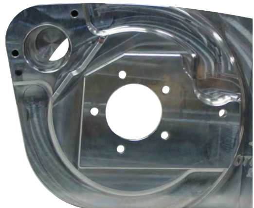
Close-up detail of starter location and hidden ring gear design.
