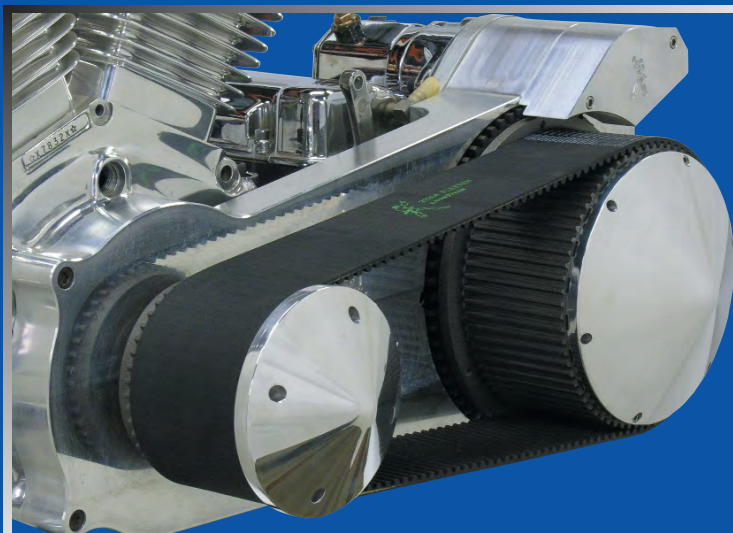
16440 & 16443 INTIMIDATOR 3.0" primary belt drive with optional 40096 'Hubcap' front pulley cover and 40099 'Hubcap' rear pulley cover
